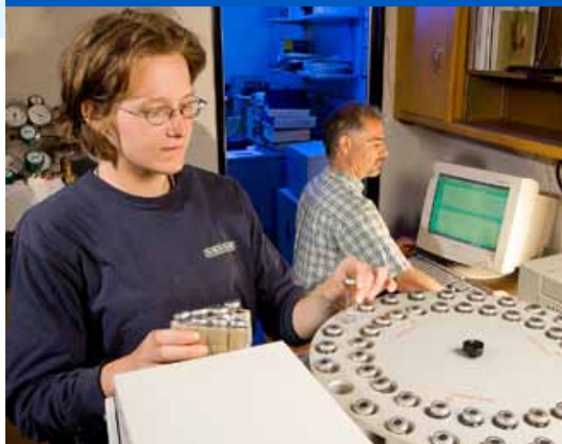
University of Minnesota technician Sonya Ewert (left) and ARS soil scientist Rodney Venterea use a gas chromatograph to determine amounts of greenhouse gases in samples collected from fields.
