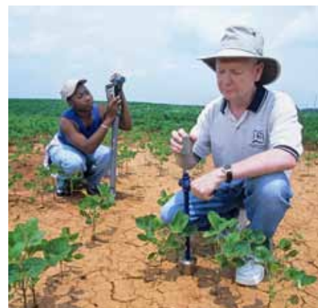
ARS hydrologist Tom Jackson and student Parmecia Jones use different methods to test soil moisture. The measurements will be compared to see which more accurately validates data obtained via satellites.
