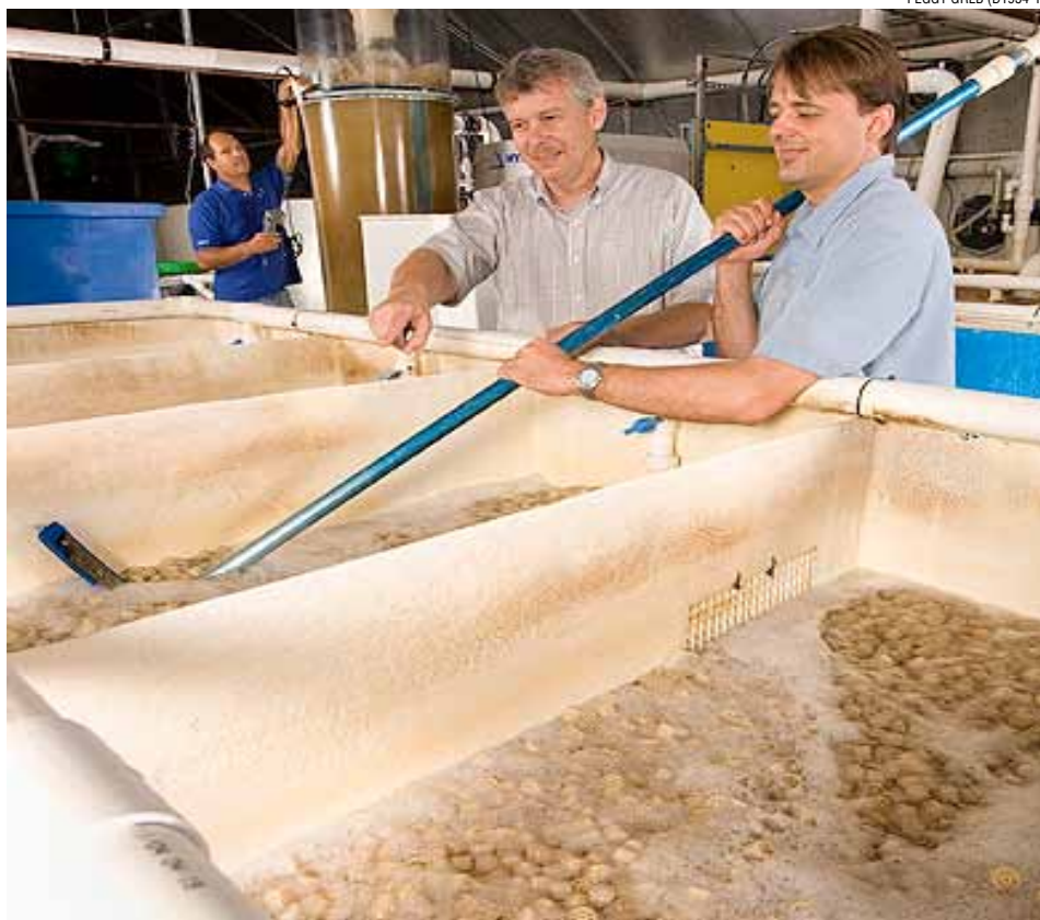
At the Florida Atlantic University/Harbor Branch Oceanographic Institute, Todd Lenger (right) and professor Paul Wills maintain and adjust movement of the system's biofilter media (the small, round objects in the water). In the background, facility systems manager Richard Baptiste monitors dissolved oxygen concentration.
