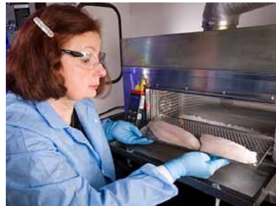
Food microbiologist Kathleen Rajkowski places a frozen catfish fillet into a device for surface decontamination by pulse UV treatment.
