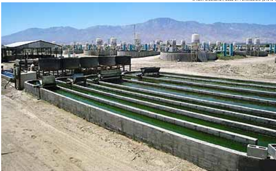
Microalgae grown in raceways at Kent BioEnergy, in San Diego, California. The microalgae will be used in a variety of applications.
