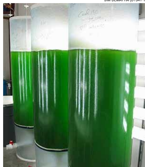
Containers of algae cultures at the Carbon Capture Corporation in Calipatria, California. The algae will be used to inoculate large production ponds.
