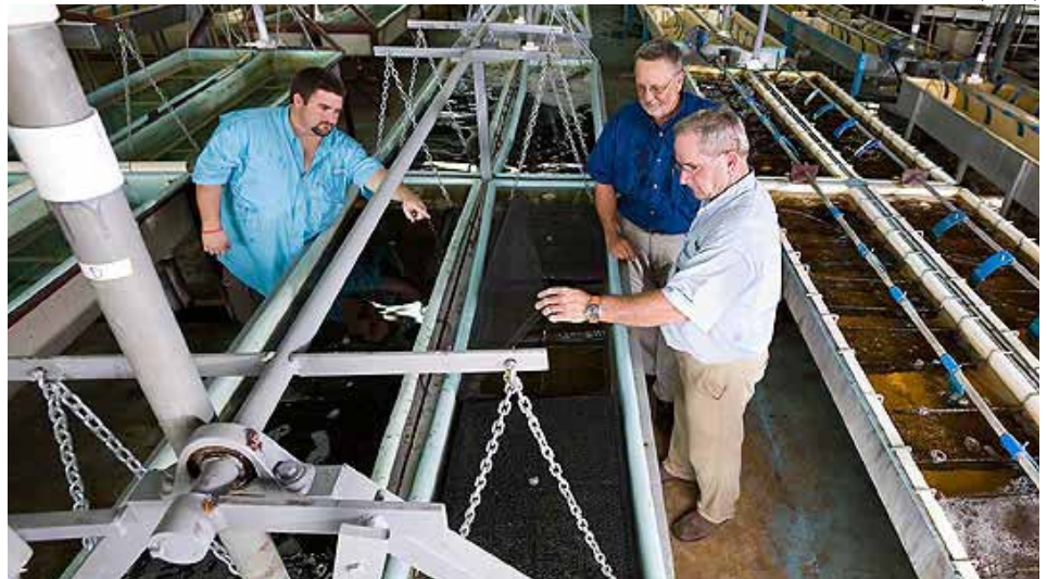
Catfish farmer Bobby Jones (left) and his father Robert A. "Shorty" Jones, of Needmore Fisheries LLC, observe the "see-saw" egg incubator with co-developer fish biologist Les Torrans (center). The two farmers plan to replace their traditional paddle-type incubators (seen on the right, behind Jones) with the new see-saw device before next spawning season.
