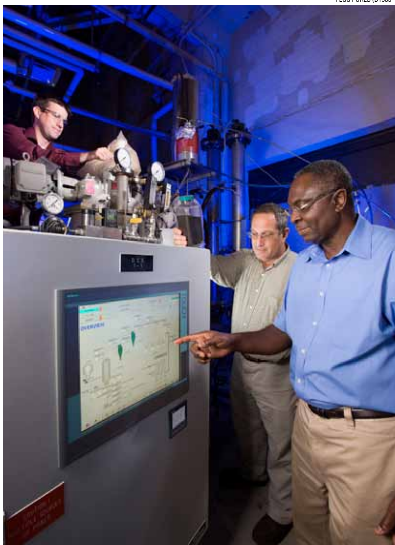
Chemical engineer Akwasi Boateng (right) and mechanical engineer Neil Goldberg (center) adjust pyrolysis process conditions while chemist Charles Mullen (left) loads the reactor with bioenergy feedstock.
