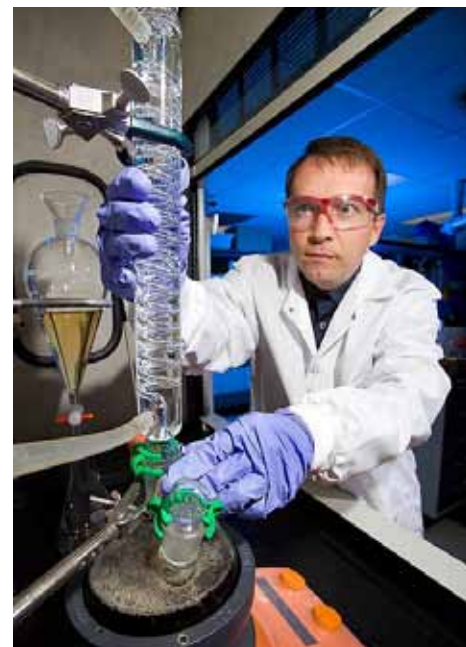
ARS chemist Bryan Moser uses a reflux condenser to produce field pennycress biodiesel.
