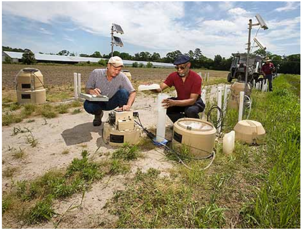
ARS soil scientist Ray Bryant (left) and UMES associate professor Arthur Allen collect samples of groundwater before and after it is filtered through an underground “curtain” of gypsum. The low-cost gypsum curtains remove phosphorus from the groundwater before it flows into a drainage ditch, preventing the phosphorus from reaching the Chesapeake Bay.
