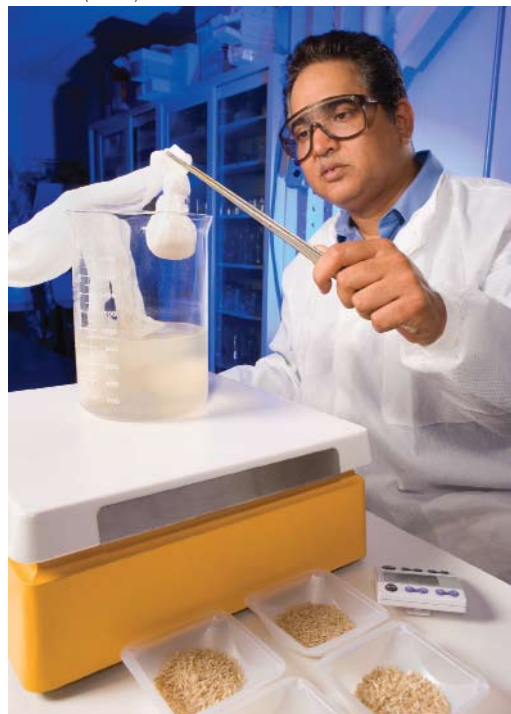
Food technologist Harmeet Guraya tests the cooking time of different brown rice varieties. Guraya developed a patented treatment that reduces the cooking time of brown rice to 20 minutes.
