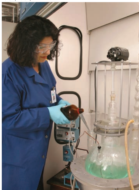
At the NCAUR lab in Peoria, chemist Sevim Erhan (now center director at the Eastern Regional Research Center in Wyndmoor, Pennsylvania) formulates a biodegradable lubricant using an ARS patented biobased antiwear additive.
