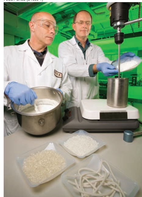
Food technologist Artur Klamczynski (left) and plant physiologist Greg Glenn prepare batches of starch-based dough which will be further processed by extrusion to form heat-expandable pellets.
