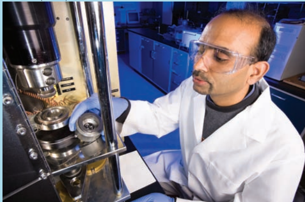
Visiting chemist Brajendra Sharma uses a standard four-ball test method to measure friction and wear properties of vegetable-oil-based antiwear additives. The additives can be used in either biodegradable or conventional lubricants and greases.
