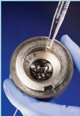
Close-up of the additive being placed onto ball bearings before friction test at right.
