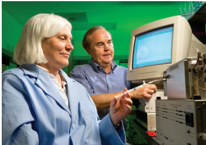
Technician Sue Wise and microbiologist Vince Varel use a gas chromatograph to measure the amount of methane, a greenhouse gas, in manure from cattle fed wet distiller's grains.
