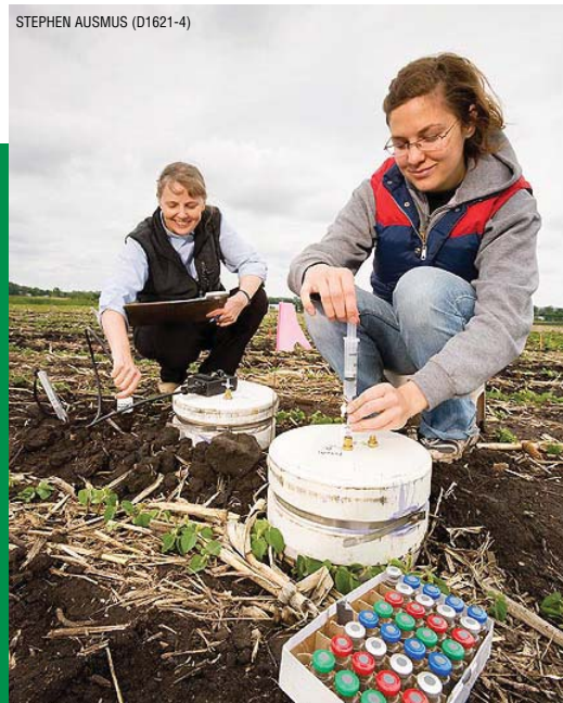
Using closed vented chambers, biological science aide Rochelle Jansen (right) and soil scientist Jane Johnson collect gas emissions from soil. Samples will be analyzed for carbon dioxide, nitrous oxide, and methane with a gas chromatograph.
