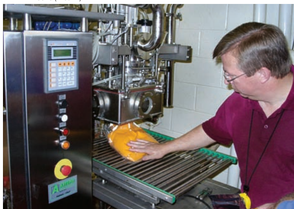
In a pilot plant at North Carolina State University, plant coordinator Gary Cartwright oversees the testing of aseptic packaging of sweetpotato puree using rapid microwave processing.
