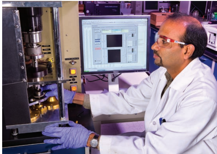
Visiting chemist B.K. Sharma measures friction and wear of soy-based oil for use in Alcoa's metalworking fluids.
