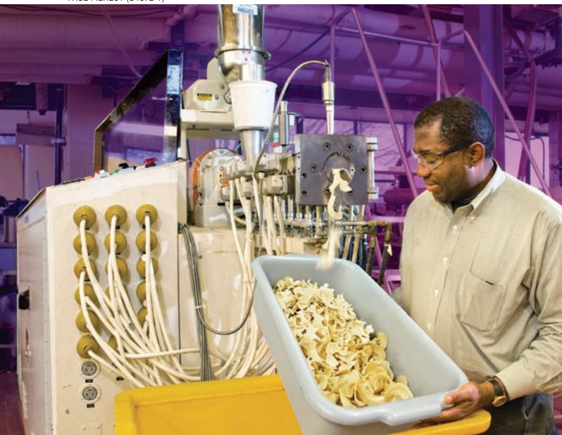
At the Eastern Regional Research Center in Wyndmoor, Pennsylvania, food technologist Charles Onwulata processes texturized whey proteins with a twin screw extruder to make healthy snack products.
