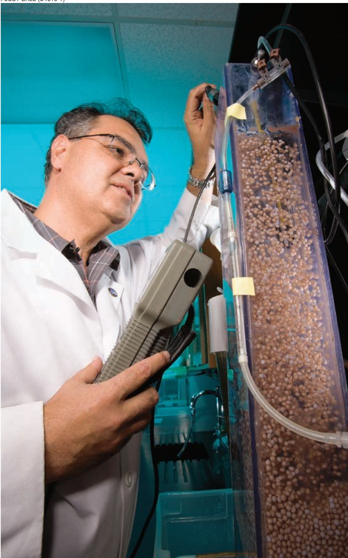
Soil scientist Matias Vanotti monitors conditions in a bioreactor that uses immobilized bacteria to remove nitrates from agricultural effluents.
