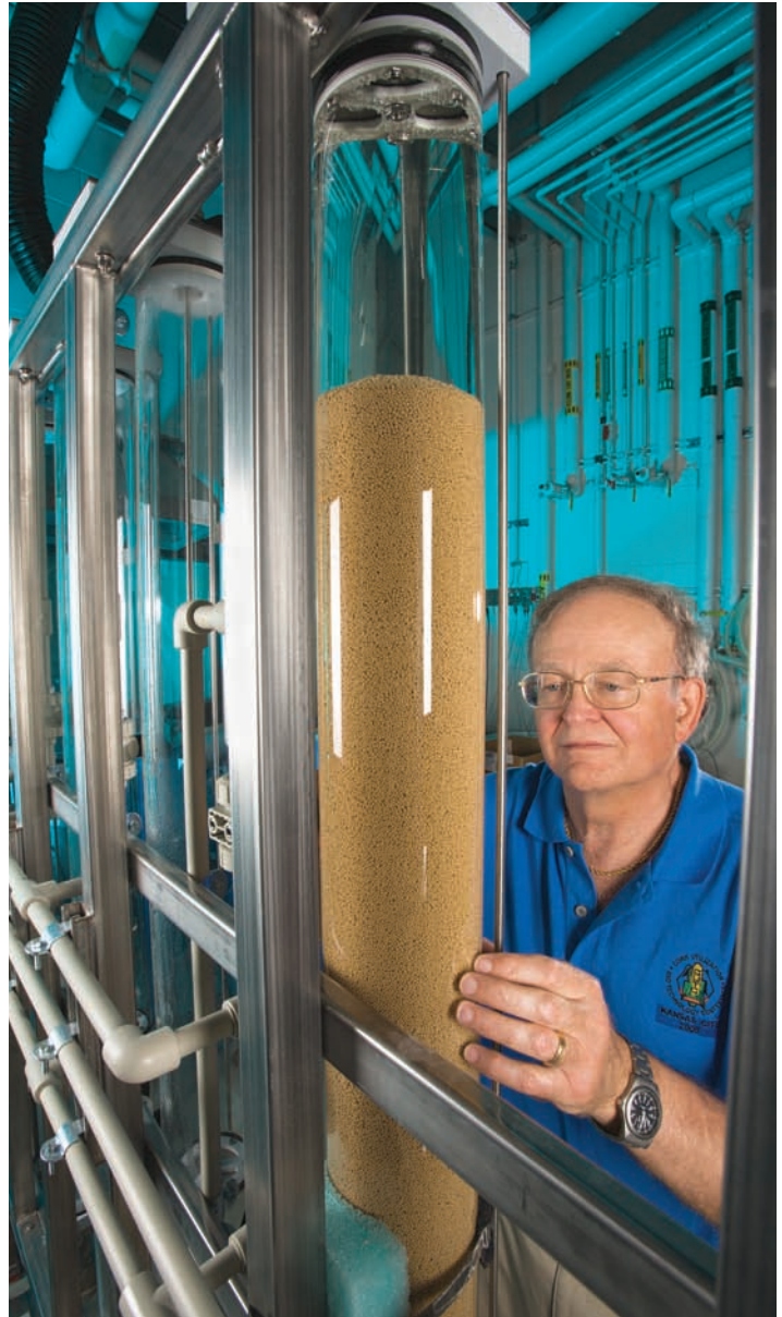
David Sessa, a chemist in the ARS Plant Polymer Research Unit, is checking for air bubbles in a chromatographic column to be used for decolorizing and deodorizing yellow zein solutions. Sessa is co-designer of the multicolumn apparatus for pilot-scale operation.
