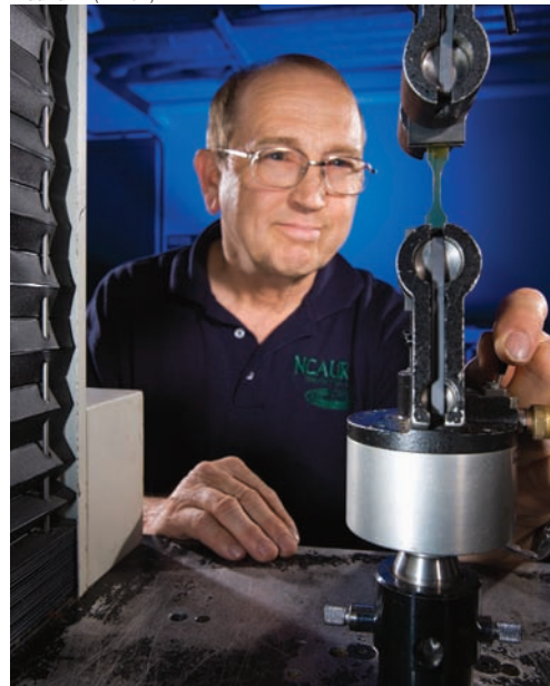
Using an Instron universal testing machine, technician Gary Kuzniar evaluates the mechanical properties of a tensile bar from chemically modified zein.
