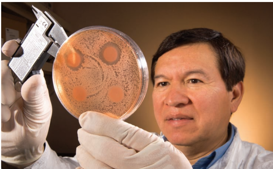
Two antimicrobial edible film disks (the top two in the petri dish) repel E. coli O157:H7 growth in the agar surrounding them. Roberto Avena-Bustillos, a collaborating researcher from the University of California-Davis, uses a micrometer to measure the width of the clear agar zone around one of the two disks. The bottom two disks are controls.
