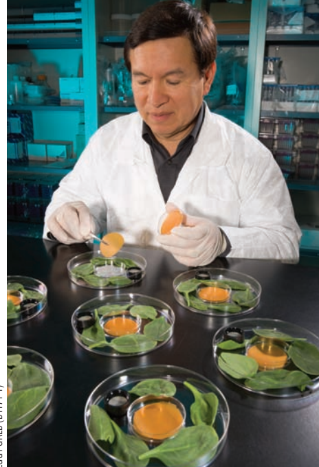
Roberto Avena-Bustillos places an antimicrobial edible film into a small dish within a larger dish of spinach leaves inoculated with E. coli O157:H7. The larger dish is then sealed to evaluate the efficacy of antibacterial vapors released from the film.
