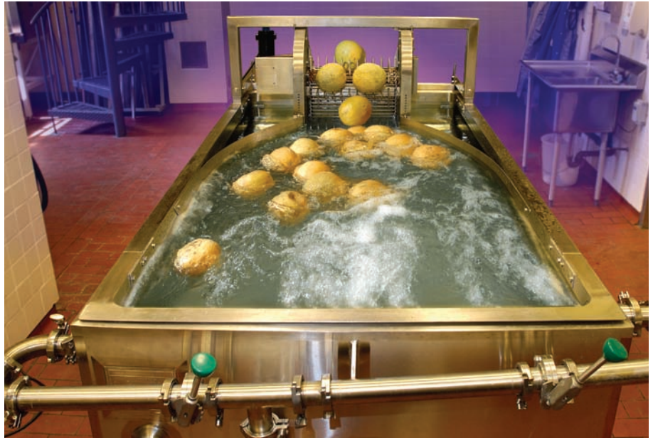
Surface pasteurization of cantaloupes using a commercial-scale dump tank (designed at ARS's Eastern Regional Research Center) in ERRC's biosafety level-2 pilot plant.
