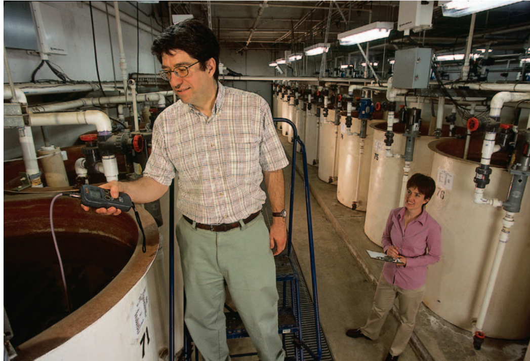
In a large room located under the sand tanks are 24 reservoirs containing about 2,000 liters of varying-strength saline solutions used to irrigate test plants. Don Suarez, salinity laboratory director, and Christy Carter measure and record pH and electrical conductivity.
