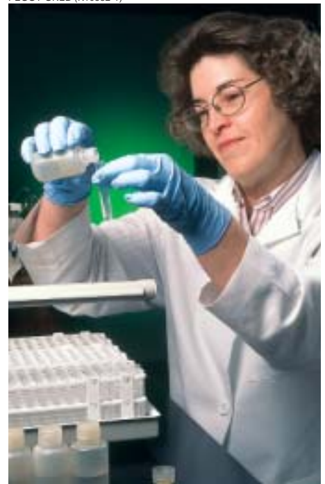
Physical science technician Jeanette Herring uses a flow-injection analyzer to determine nitrogen and phosphorus concentrations in manure and runoff.
