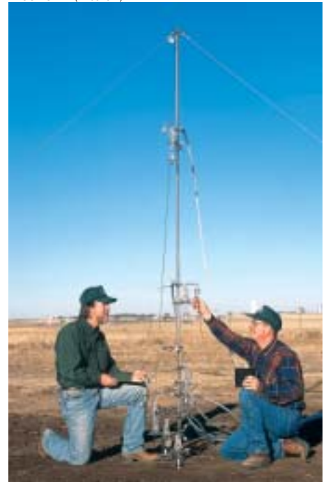
As part of ammonia emission studies, soil scientist Richard Todd (left) and biological science technician Larry Fulton measure air flow rate through ammonia collectors installed on a simulated feedlot surface.
