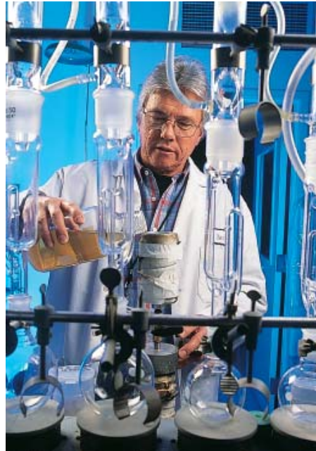
Technician Steve Vinyard pours guayule resin into a pressure treatment chamber that impregnates wood with the termite-repelling liquid.
