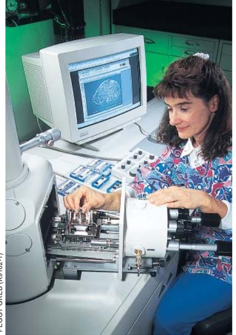
**ARS technician Leona Horst loads a fuchsia leaf sample into the variable-pressure scanning electron microscope.**
