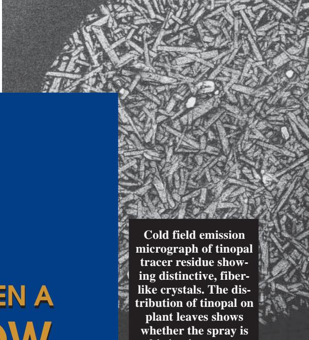
Cold field emission micrograph of tinopal tracer residue showing distinctive, fiber-like crystals. The distribution of tinopal on plant leaves shows whether the spray is hitting its target.
