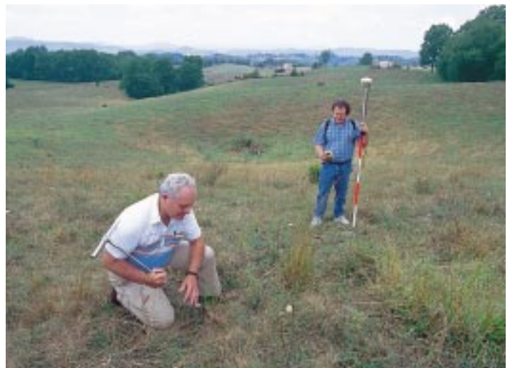
In studying animal waste distribution in a karst sinkhole, plant physiologist Ralph Clark (left) withdraws a soil sample while hydrologist Doug Boyer operates a global positioning system device.
