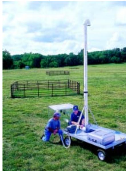
**Plant physiologist Howard Skinner (right) demonstrates the plant canopy photosynthesis system to farm operator Glenn Moyer. It pumps carbon dioxide into the Plexiglas chamber, which is placed over a selected area of pasture to see how much is absorbed by pasture grasses. The grazing exclosures in the background are used to study grazed and nongrazed pastureland.**
