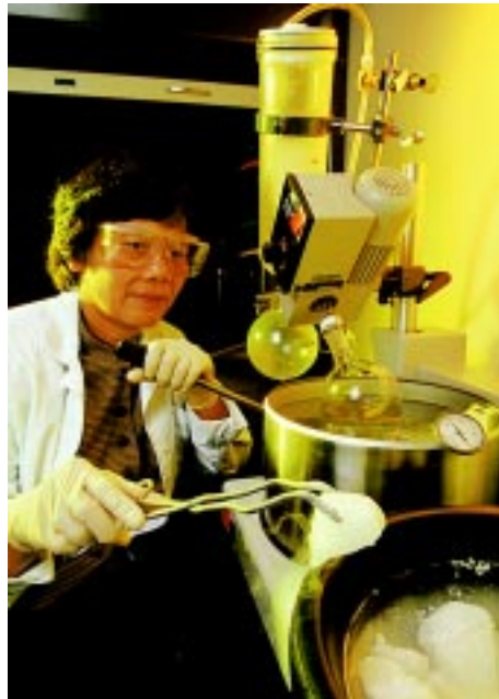
Chemist Perla Schmidt uses a rotary evaporator to remove solvent from lipids extracted from volunteers' blood samples. She is putting dry ice in the top of the evaporator to cool and condense the solvent for removal.
