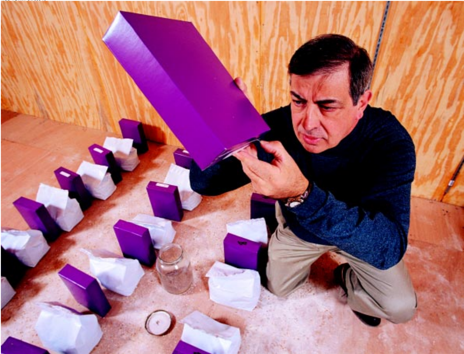
Entomologist Mike Mullen checks seals for signs of infestation after a 3-month test of consumer-size packages.
