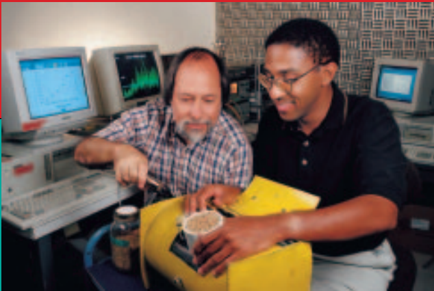
After ARS entomologist Richard Mankin (left) inserts a sensitive microphone into the grain sample container, engineering technician Everett Foreman will place them both in a sound-insulated cylinder that allows the chewing sounds of insects to be detected and amplified. (K7361-1)
