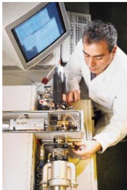
Using high-performance liquid chromatography, chemist Frederick Khachik analyzes an extract of human blood for dietary carotenoids and their metabolites. (K7496-1)
