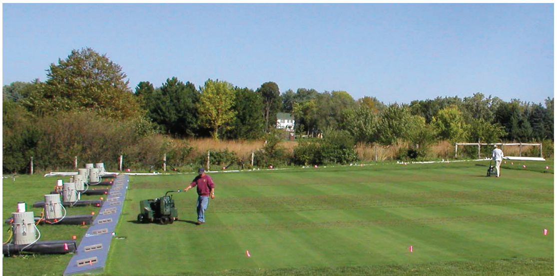
Core cultivation of plots. Some plots were cultivated with solid tines, others with hollow tines. Runoff was collected from plots cultivated by each method and analyzed for pesticide and fertilizer (nitrogen and phosphorus) content.
