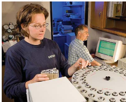
University of Minnesota technician Sonya Ewert (left) and ARS soil scientist Rodney Venterea use a gas chromatograph to determine amounts of greenhouse gases in samples collected from the field.
